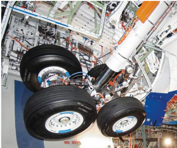
Landing gear testing... (A380 @ 12 mio. cycles)
